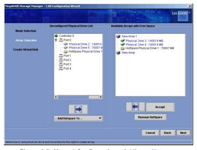
Figure 6-7: Manual Configuration - Adding a Hotspare
